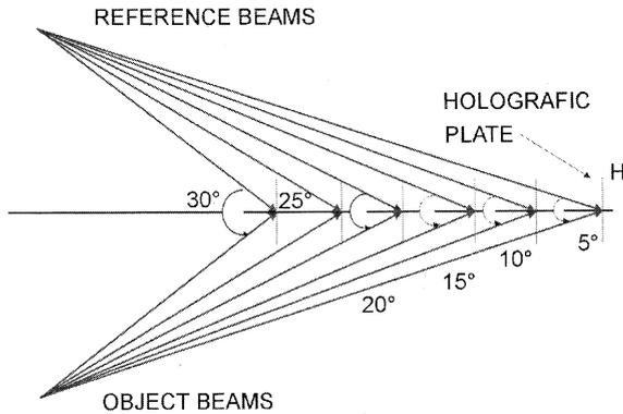
Fig. 4. Experimental configuration employed to make diffraction grating, changing the interference angle between the beams.
