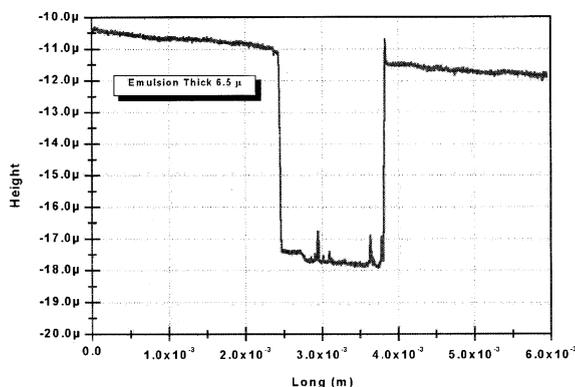
Fig. 3. Thickness of the emulsion, with approximate margin of error  $0.25 \mu\text{m}$ , which to measure oneself with Surfalyzer 4000.
