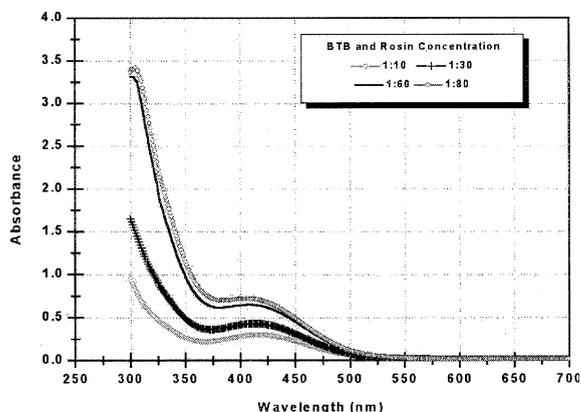
Fig. 2. Shows the absorbance spectrum curves versus wavelength for different concentration of BTB and rosin. In the UV region this material corresponds a higher absorbance.
