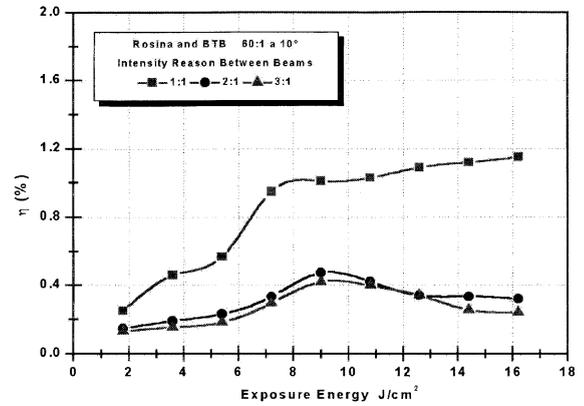
Fig. 11. Diffraction efficiency versus exposure energy in function of the intensity reason between the beams, to obtain the 1:1 reason the better.
