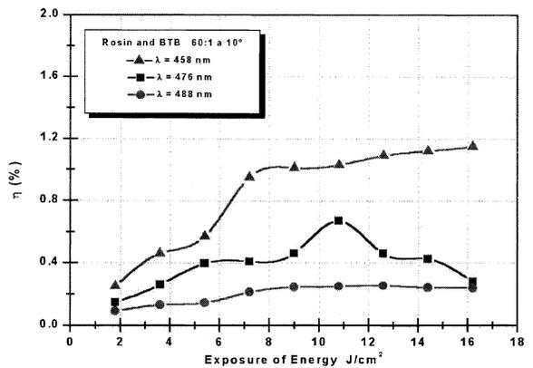
Fig. 12. Diffraction efficiency versus exposure energy, influence of color ( $\lambda$ ). Diffraction grating record with the next wavelength  $\lambda = 457, 476$  and 488 nm where the material in the blue color  $\lambda = 457$  nm is more photosensitive.
