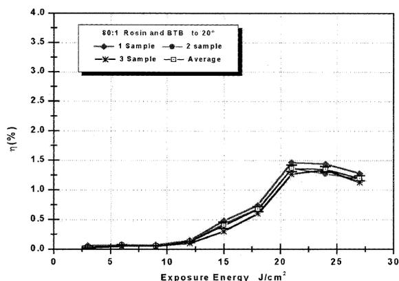
Fig. 8.  $\eta$  (%) reproductions of the gratings to obtain margin of error and average for 80:1 concentration to obtain the 1.5% of  $\eta$  to exposure energy bigger and 1.35% the average.
