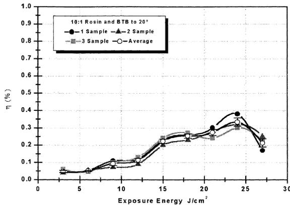
Fig. 5.  $\eta$  (%) reproductions of the gratings to obtain margin of error and average for 10:1 concentration where to low  $\eta$  the order 0.4% as maximum and 0.33% the average.
