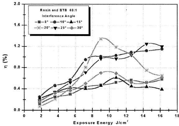
Fig. 10. Diffraction efficiency versus exposure energy changing the interference angle between beams, showing the bigger  $\eta$  (%) for the 10° angle.
