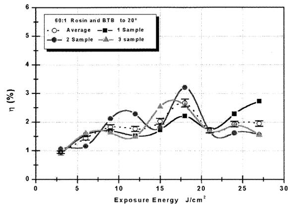
Fig. 7.  $\eta$  (%) reproductions of the gratings to obtain margin of error and average, for 60:1 concentration to support a soft increase in your  $\eta$  (%). Having 3.25% of  $\eta$  maximum and 2.6% the average.
