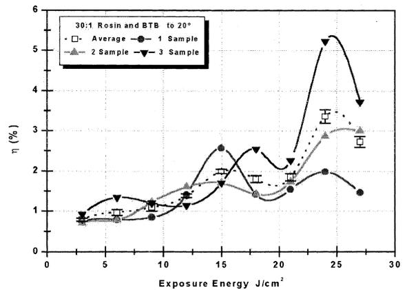
Fig. 6.  $\eta$  (%) reproductions of the gratings to obtain margin of error and average for 30:1 concentration. Showing 5.3% of  $\eta$  maximum and 5.3% the average.
