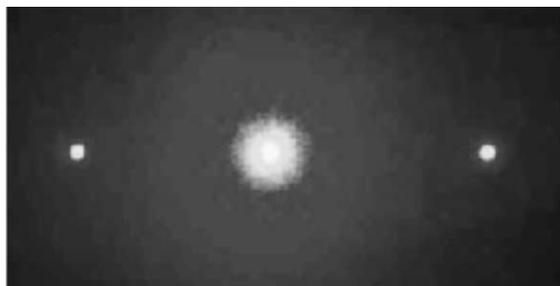
Fig. 14. Diffraction efficiency pattern of the grating of BTB and rosin, with 60:1 concentration and with 2.76% of  $\eta$  showing the 0, +1 and -1 orders.
