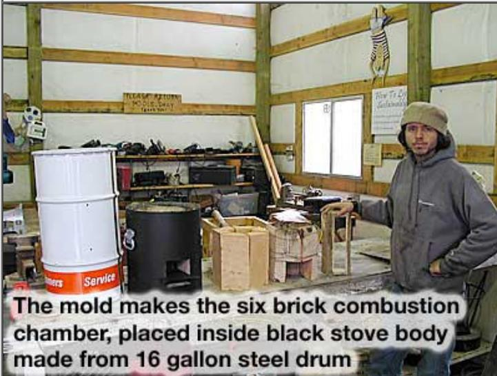
**The mold makes the six brick combustion chamber, placed inside black stove body made from 16 gallon steel drum**
