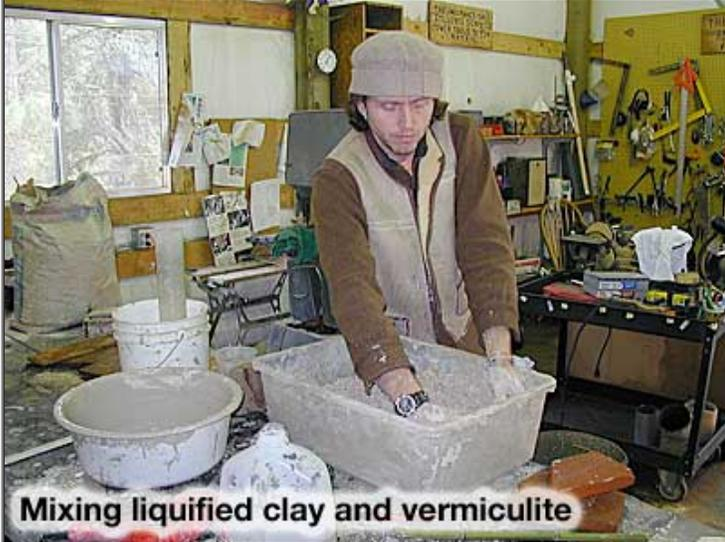
**Mixing liquified clay and vermiculite**
