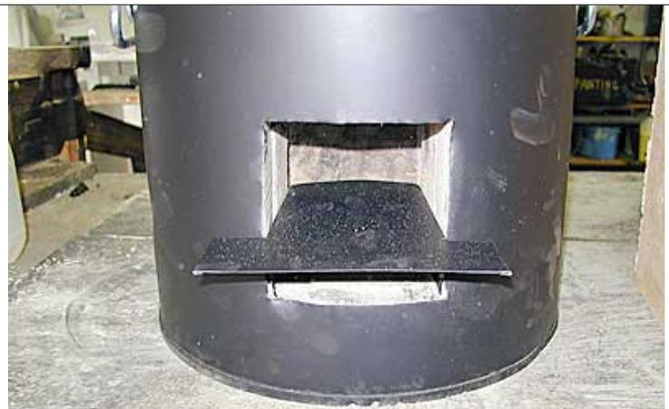
**A shelf holds burning sticks of wood above the floor of the combustion chamber**
