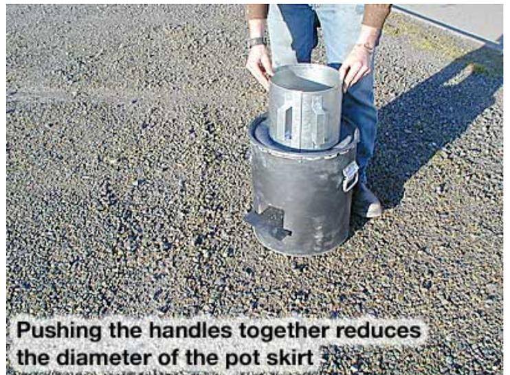
**Pushing the handles together reduces the diameter of the pot skirt**
