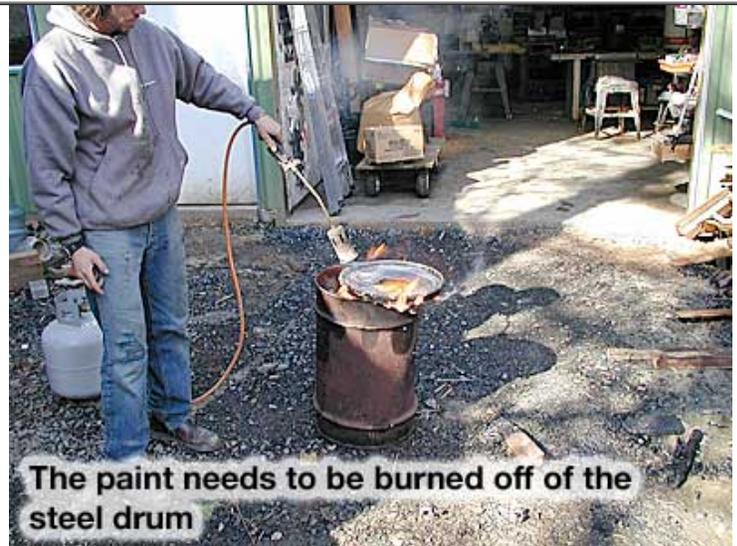
**The paint needs to be burned off of the steel drum**
