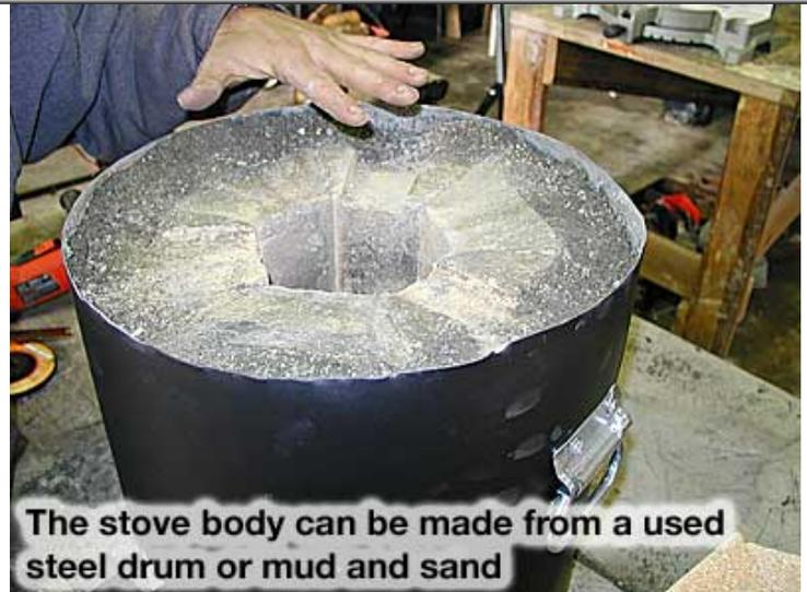
**The stove body can be made from a used steel drum or mud and sand**
