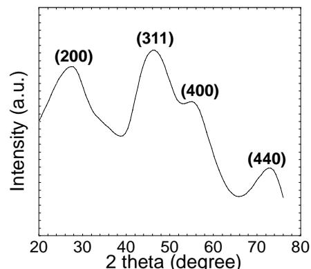
**Figure 3.** XRD scan of iron oxide nanoparticles.
