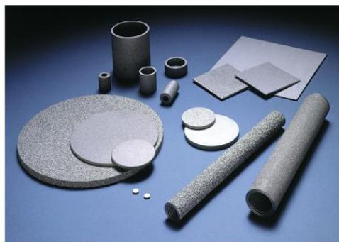
Gravity sintered parts have certain restrictions-for example, some draft must be allowed on longer parts-there is a 1 percent taper minimum-and certain advantages- i.e. low tooling cost, ability to make cones and tapering sections and undercuts.
