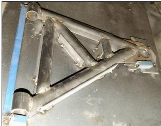
Which brings us to the next point regarding jigs. Jigs are very often used when things need to be held in the right positions for welding. Especially if the person building the object is not the one who will be doing the welding, a jig ensures accuracy and location. If the jig is strong enough, it can also prevent distortion that almost inevitably occurs during welding. But that requires a very rigid jig – most jigs are for positional location rather than to prevent distortion.
