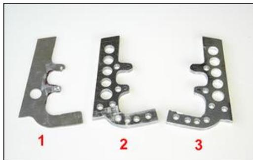
Here's another example, this time the front suspension upright of a human-powered vehicle. In addition to supporting the stub axle, the upright had to locate and support the hydraulic brake caliper. This required absolute accuracy in the hole locations - a template (1) was a necessity. It was used to form the right-hand upright (2) and then by a mirror image reversal, the left-hand upright (3).
