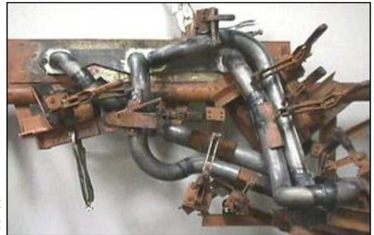
But instead the prototype is used to make a jig.
