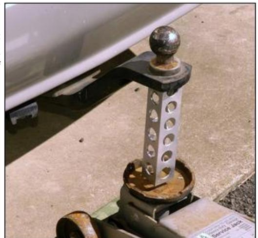
Incredibly, this section of lightweight, drilled square aluminium tube can support about half the weight of the car! (Note the rear wheels off the ground.) Ahh, but what about in bending? That's a much tougher ask.
