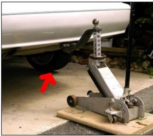
This time, the test piece was supported on two jack-stands beneath the raised towbar. In this position, the rear wheels are off the ground. The jack was then lowered until...
