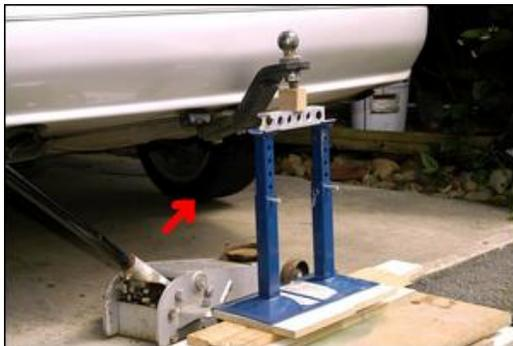
...the rear weight of the car rested fully on the test piece. Incredibly, again the 150g aluminium tube supported the load! (Again note the rear wheels off the ground.) But was the tube bending like a banana?
