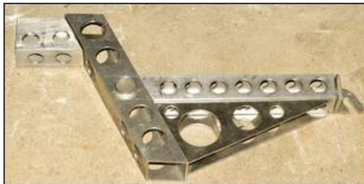
Talking about tube, the strength of the material (especially in bending) goes up very quickly with increases in depth or diameter. In other words, a 50mm tube is **much** stronger than a 25mm tube, even with both having the same wall thickness.
