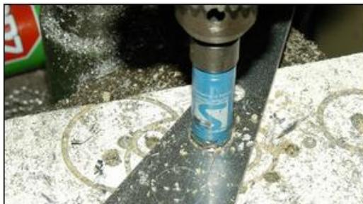
The next step is to drill right through with the pilot drill. After doing this, spray some lubricant on the hole-saw and material – with aluminium, a penetrating lubricant like RP7 or WD40 (where do they get these names from?!) works well. Then cut the hole, lifting the hole-saw frequently to clear swarf and lubricating as necessary. A chattering saw blade will give a poor result, and in extreme cases the resulting hole will not be round. If you are drilling through sheet, make sure you place a
