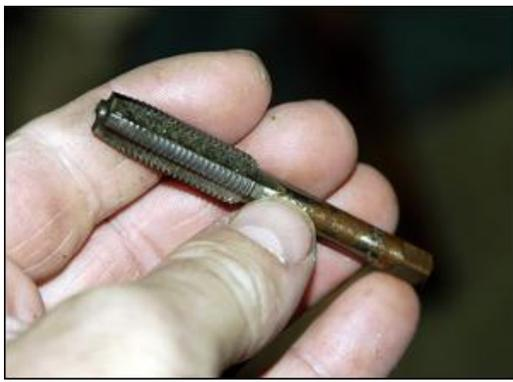
clearance slots) and the thread is formed with a sharp cutting edge. In brief (we'll cover the use of the tool in more detail below), a hole of the correct diameter is drilled in the material and then the tap used to form the internal thread in the hole.
