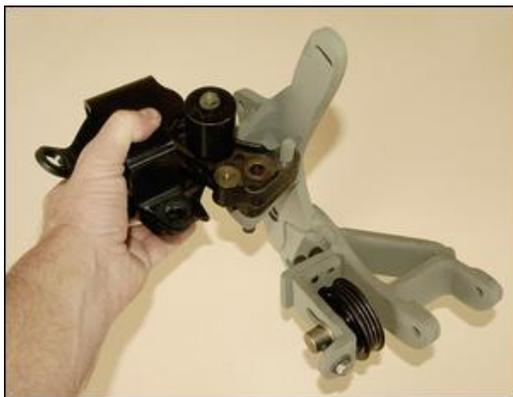
Take this supercharger bracket I made. The bracket incorporated a belt idler pulley and it was important that the flanged pulley was adjustable so it could be set at exactly 90 degrees to the surface of the belt. That meant it had to be bolted into place not welded – loosen the bolts and the pulley could be adjusted.
