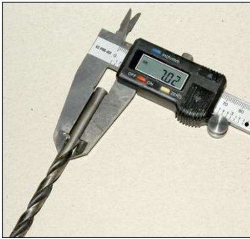
quick, easy and accurate) to measure the actual size of the shank. Creep up to the correct hole size in a number of steps by using a succession of increasing size drills. In this way, the final hole size will be more accurate. Make sure that you are drilling at right-angles to the work – it is preferable to use a drill press.
